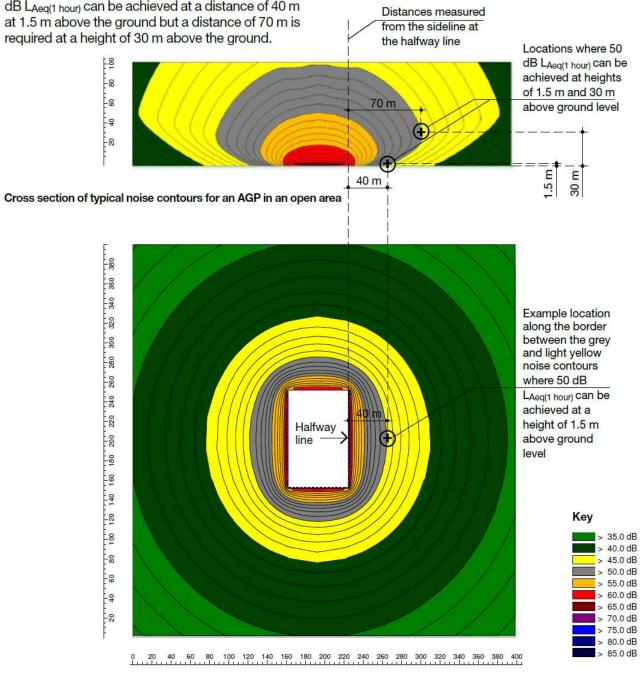
Plan of typical noise contours for an AGP in an open area measured at a height of 1.5 m above ground level
